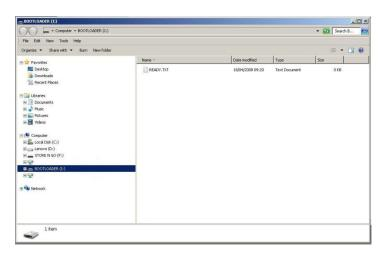
9. Open the "BOOTLOADER" folder and drag-n-drop the s19 file.
