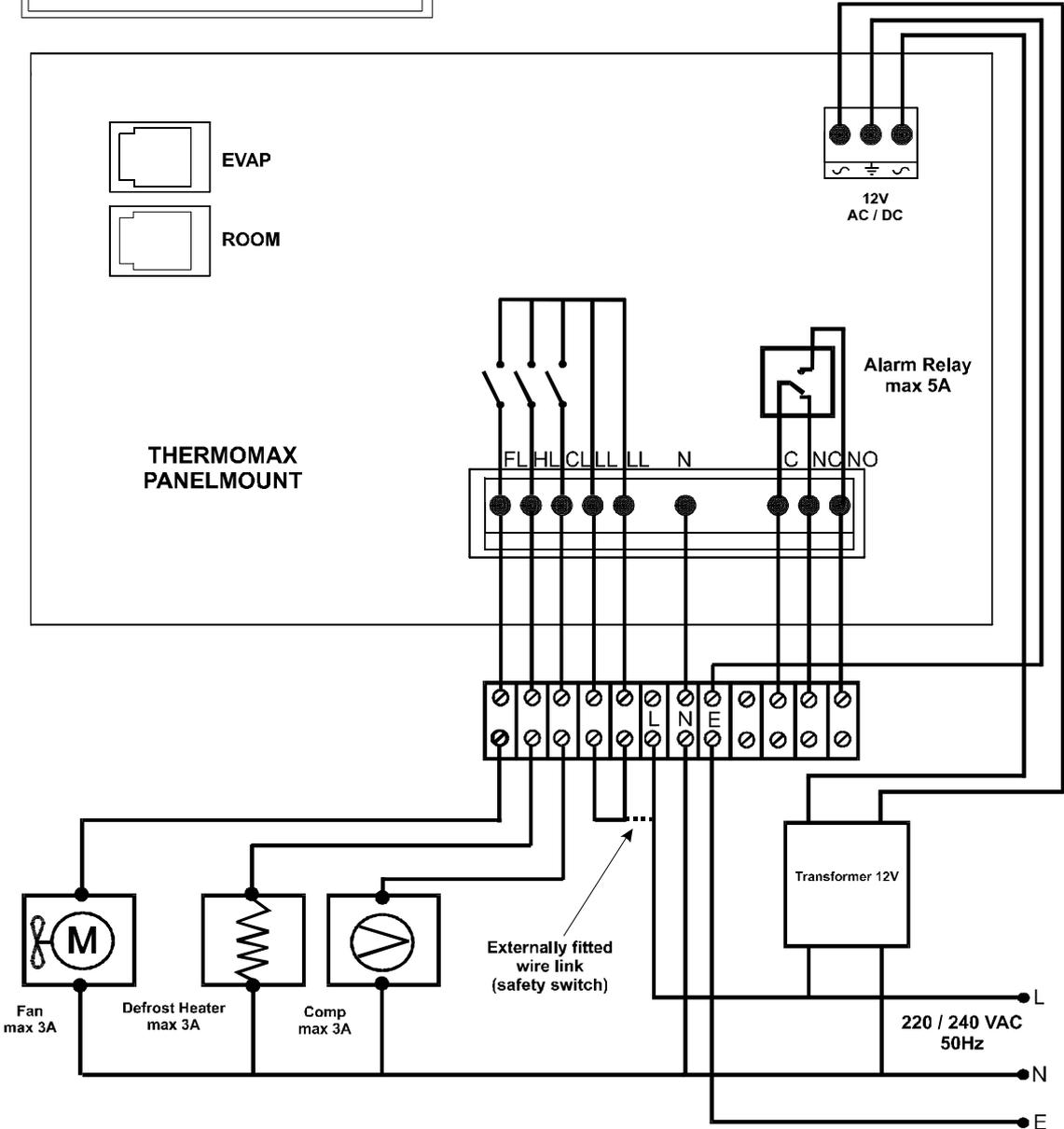
**NOTE:** The RCX 100 relay outputs should only be used to drive external contactors. They should not be connected directly to the Fan, Heater or Compressor.
