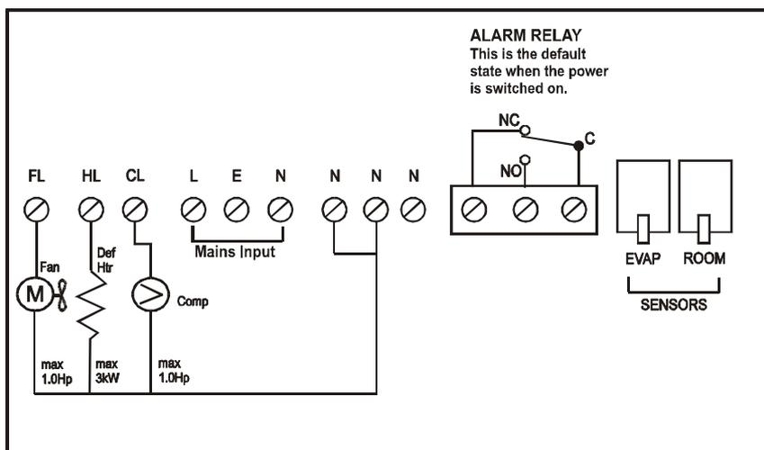
**NOTE:** If the outputs from the Compressor Live, Heater Live or Fan Live are connected to contactors, then the coil of the contactor should be properly suppressed from arcing by use of RC Suppressor modules.
