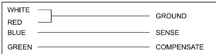
As with all PT100 sensor applications, a good connection is vital. It is therefore recommended that wherever there is any doubt, a factory-extended sensor or a sensor extender should be used.
