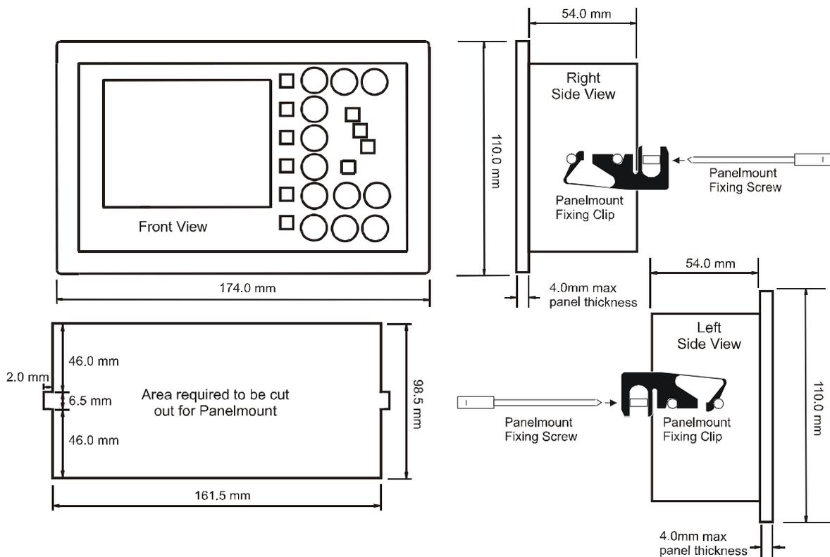
After inserting the Panelmount unit into the panel cut out, attach the two panelmount fixing clips (supplied), to the two studs at either side of the unit, (as above). The Panelmount unit is then held in place by the two Panelmount fixing screws (also supplied).
