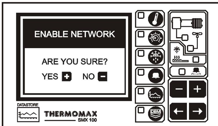
To enable the network press the
