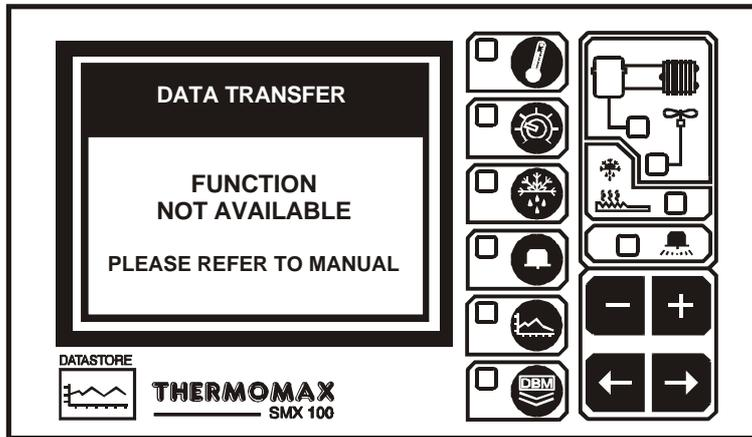
In order to download data to the Masterlink Hardware unit or print directly to a Thermomax Serial Printer, the network must be disabled.
