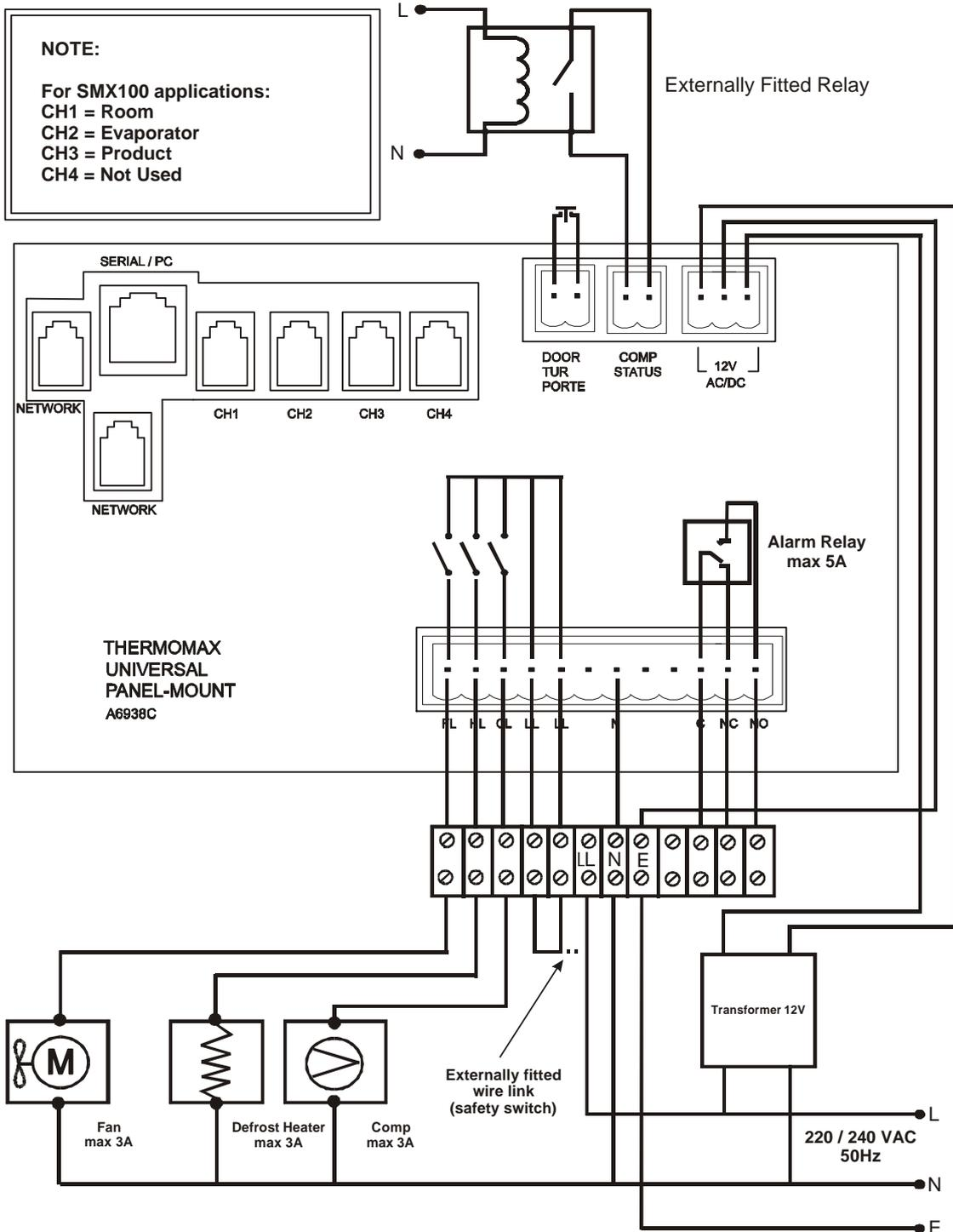
NOTE: The SMX 100 relay outputs should only be used to drive external contactors. They should not be connected directly to the Fan, Heater or Compressor.
