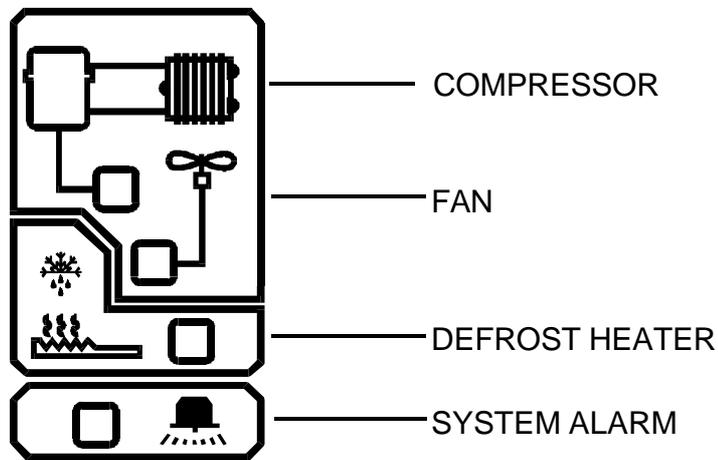
The indicators represent the state of the output relay. When lit, they indicate that the corresponding relay is energised.
