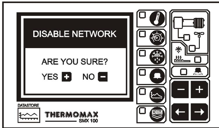
To disable the network press the **+** key. (When the **+** key is pressed, the SMX 100 will switch off and back on again).
