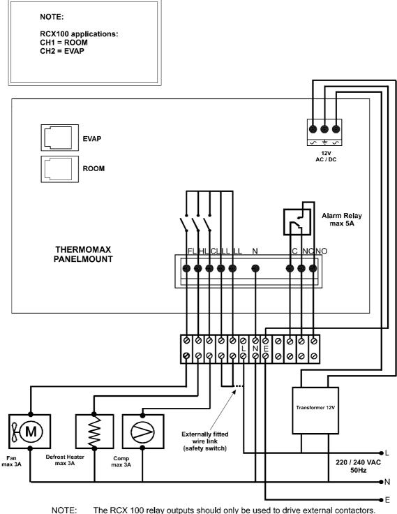
TE: The RCX 100 relay outputs should only be used to drive external contactors. They should not be connected directly to the Fan, Heater or Compressor.
